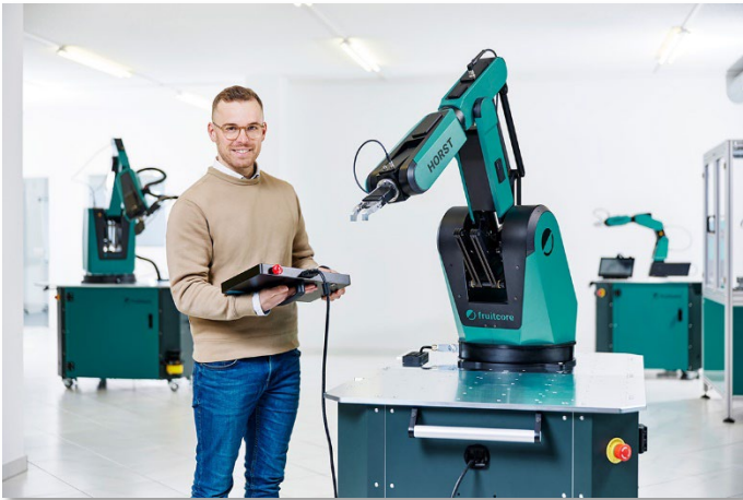
Caption: Digital Robot HORST1000, optimized by machine learning: up to 8 kg payload, 1,018 mm range, enlarged workspace.
