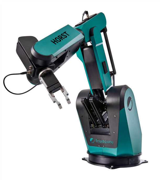
Caption: Digital Robot HORST1000, optimized by machine learning: up to 8 kg payload, 1,018 mm range, enlarged workspace.
